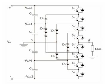
Fig. 1 Five-level NPC Inverter.
