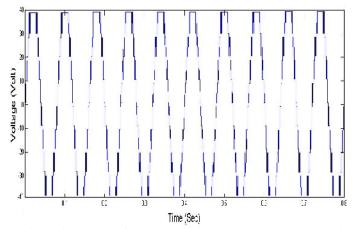
Fig. 7. Simulation result of Nine level Neutral point Clamped Multi Level Inverter.
