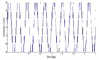
Fig. 6. Simulation result of seven Neutral point level Clamped Multi Level Inverter
